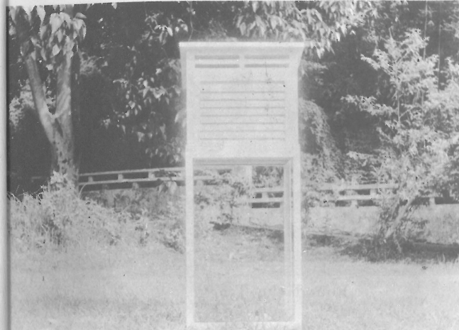
A Stevenson's Screen set up by the Geography Club for weather reporting
